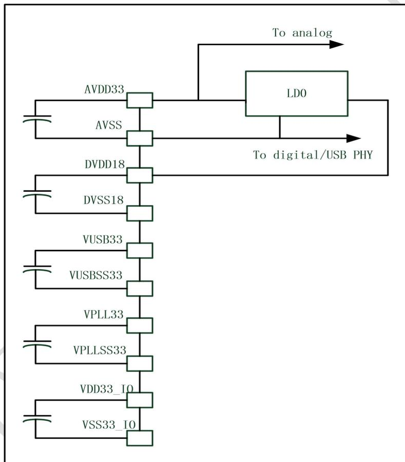
Figure 27. CJC6833A power supply diagram
