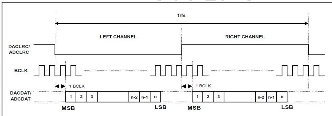
Figure 11. I2S Justified Audio Interface (assuming n-bit word length)
