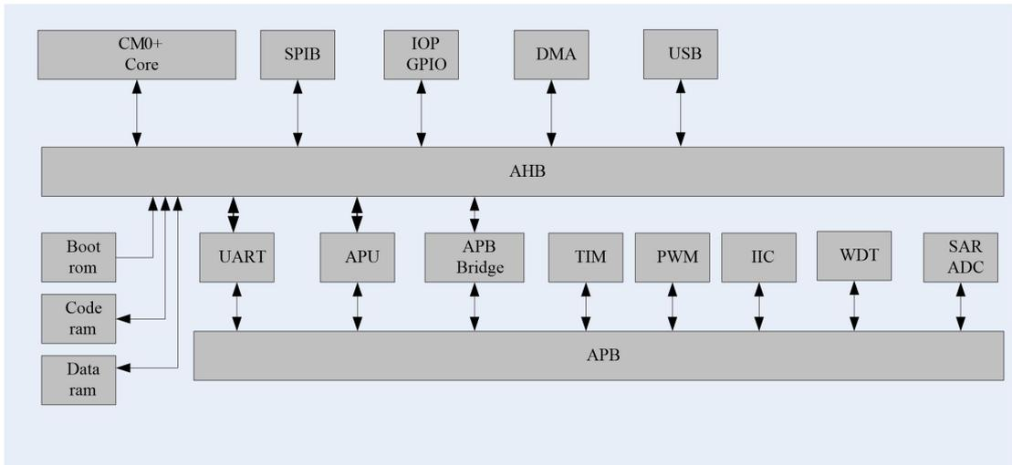
Figure 1. CJC6833A chip block diagram
