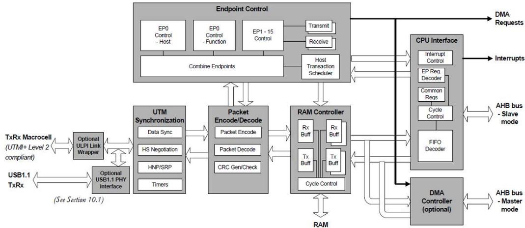
Figure 24. USB controller module block diagram
