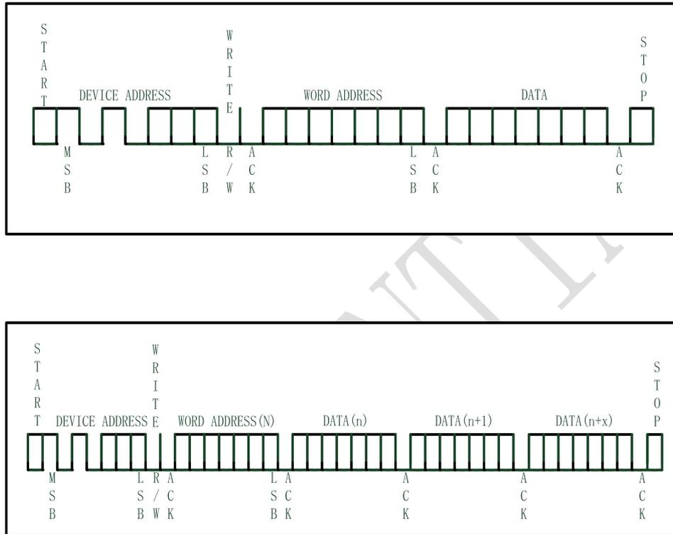
Figure 18. IIC single write and IIC burst write
