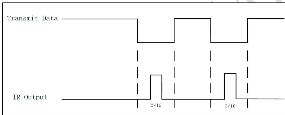
Figure 21. SIR encoding
