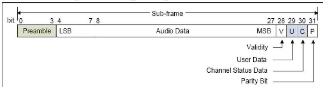
Figure 14. sub-frame structure
