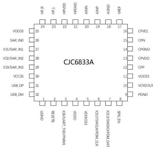
Figure 2. CJC6833A PIN diagr
