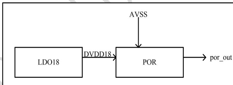
Figure 25 CJC6833A POR circuit block diagram
