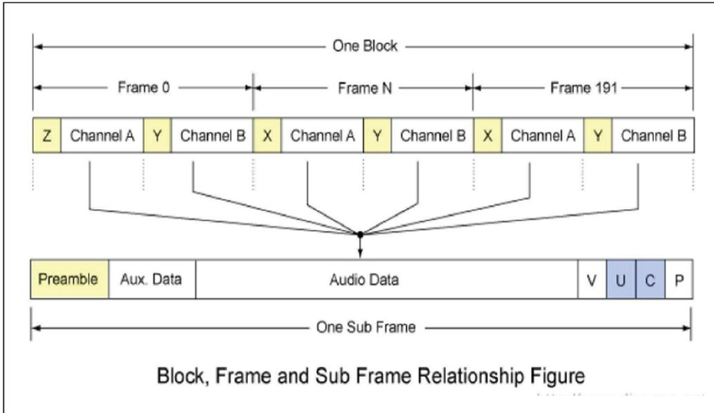
Figure 15. SPDIF block structure
