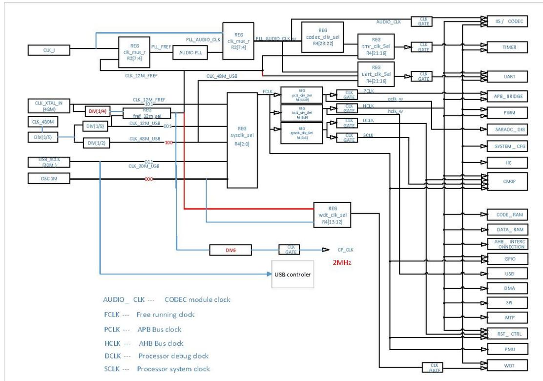
Figure 5.CJC6833A clock diagram
