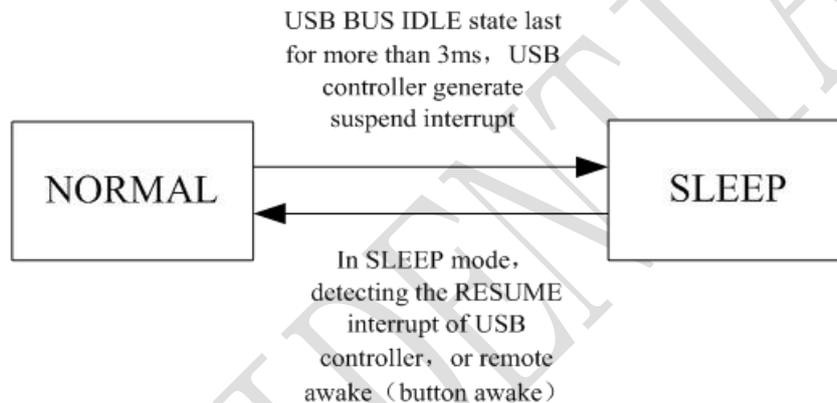
Figure 28. CJC6833A power saving mode diagram
