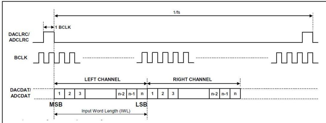
Figure 13.DSP Audio Interface (assuming n-bit word length)
