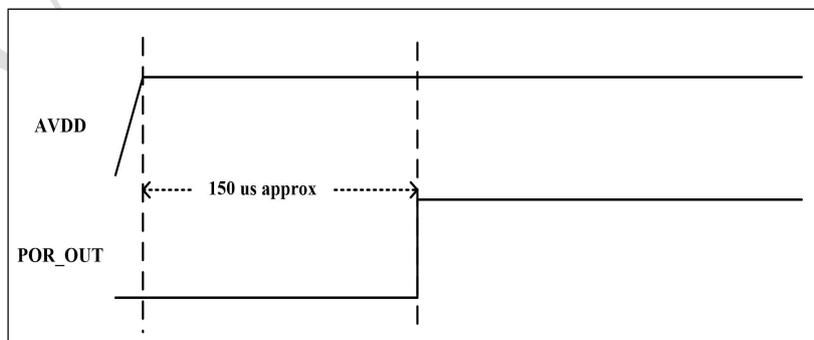
Figure 26. CJC6833A POR timing
