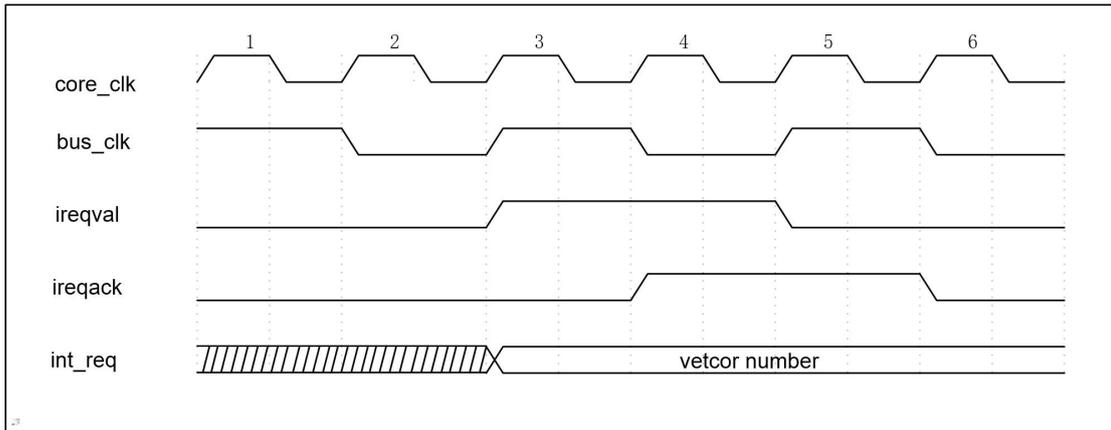
Figure 8. the interrupt REQ/ACK timing sequence diagram.
