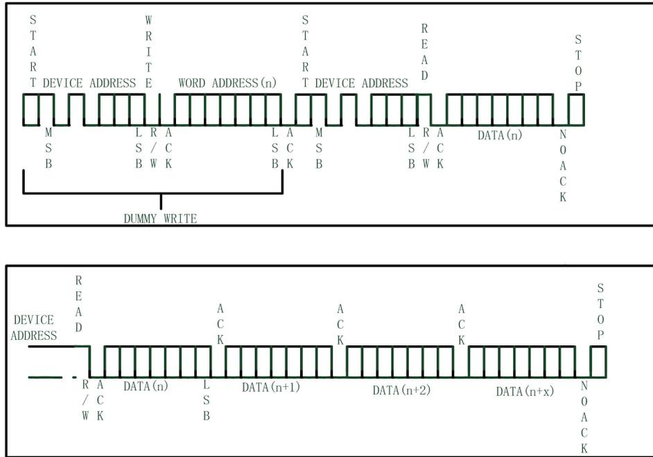
Figure 19. IIC single read and IIC burst read
