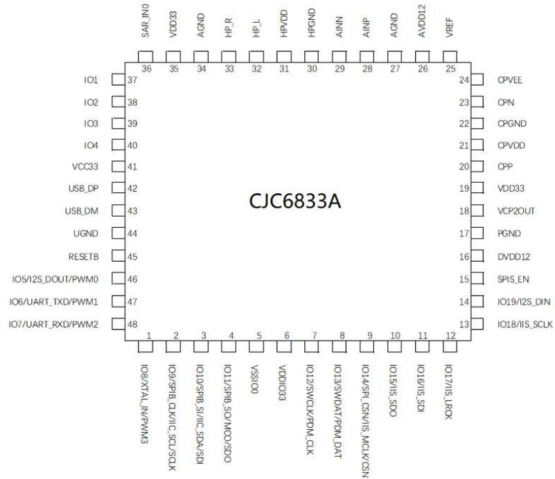
Figure 3. CJC6833A PIN diag
