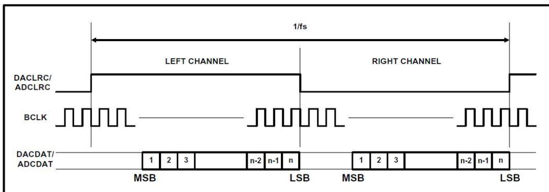
Figure 12. Right Justified Audio Interface (assuming n-bit word length)
