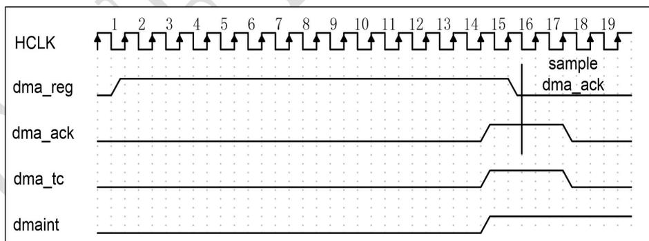
Figure 7. DMA hardware handshake mode protocol
