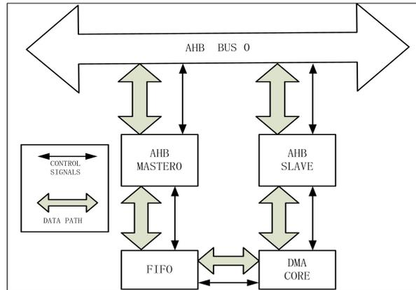
Figure 6. DMA controller module block diagram
