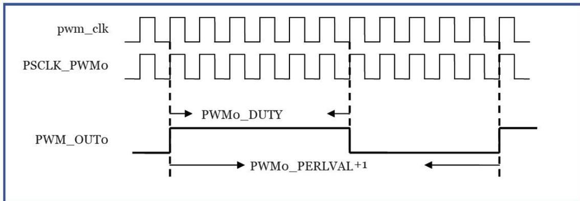
Figure 23. timing diagram of PWM
