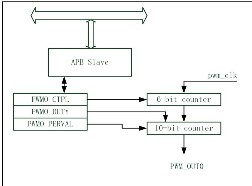
Figure 22. Block diagram of PWM
