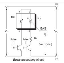
The sensor's signal should be measured during the 0.002 second Vc pulse (see *timing chart*). The numbers shown around
