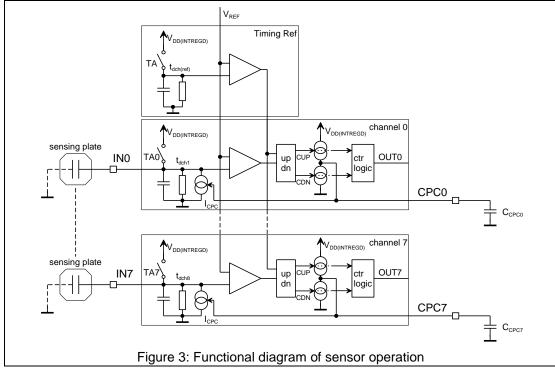
Figure 3 illustrates the functional principle of the MS8885B. The discharge times  $t_{dchx}$  on inputs INx, attached to the sensing plate capacitances, are compared to the discharge time  $t_{dch(ref)}$  of an internal RC timing element, for each sensor input sequentially. The RC timing circuits are periodically charged to  $V_{DD(INTREGD)}$  via MOS switches and then discharged via a resistor to  $V_{SS}$ . The charge-discharge cycle for each channel is governed by the sampling
