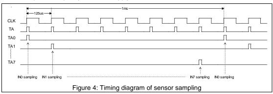
The sampling rate  $(f_s)$  is derived from the internally generated oscillator frequency. The oscillator frequency can be adjusted within a specified range by programming the CLKREG register.
