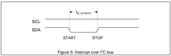
The system controller has to detect the START-STOP condition and react accordingly.
