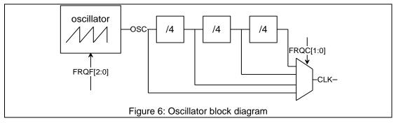
The frequency of the internal oscillator can be adjusted, and the programmable clock divider allows changing the sensor sampling rate further. This way the reaction time and power consumption of the circuit can be adjusted over a wide range.
