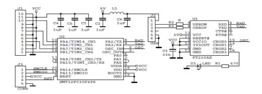
Figure 2 Circuit diagram of the SMTAS04USBmini board
