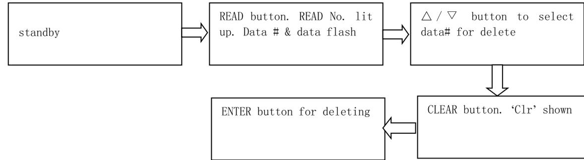
**Note:** If 'READ' button is pushed instead of 'ENTER' button, data will not be deleted and the system will directly return to the previous interface.
