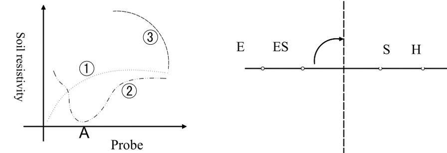
Plot 1: When depth is increased and  $\rho$  is not decreased: a bar-shaped conductor electrode is recommended.
