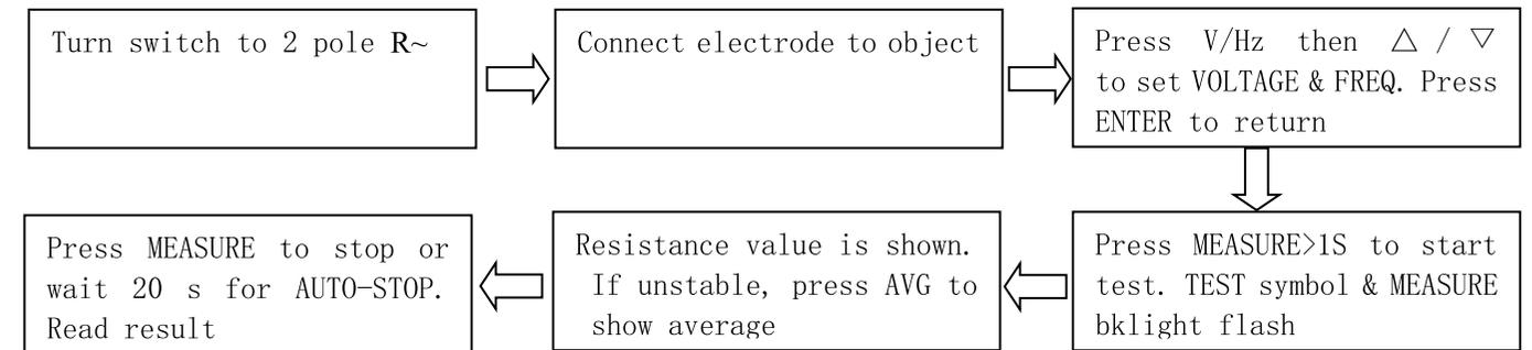
'DISPLAY' button for switching display (2 pole R~)
