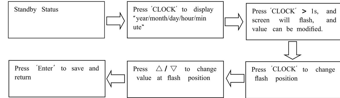
Note 1: Upon pressing the Enter button, the clock starts to run from 0 seconds.
