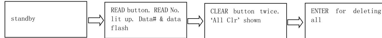
**Note:** If READ button is pushed instead of ENTER button, data will not be deleted and the system will directly return to the previous interface.
