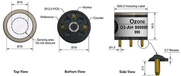
Dimensions are in millimetres (± 0.15 mm).
