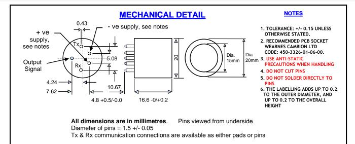
NOTE – The above pin configuration is shown for the POSITIVE version of the sensor. The NEGATIVE version has the +ve and -ve supply pin positions exchanged. See ordering details.
