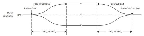
Figure 25. Fade-In and Fade-Out Operations
