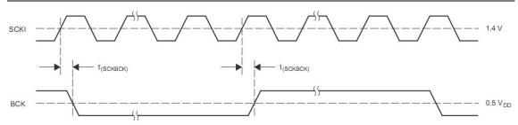
Figure 6. Audio Clock Interface Timing (Master Mode: BCK Works as Output)
