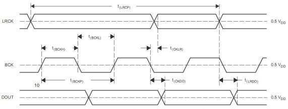
Figure 5. Audio Data Interface Timing (Master Mode: LRCK and BCK Work as Outputs)
