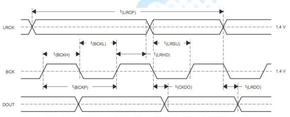
Figure 4. Audio Data Interface Timing (Slave Mode: LRCK and BCK Work as Inputs)
