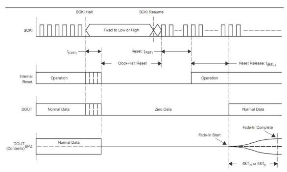
Figure 3. Clock-Halt Power-Down and Reset Timing
