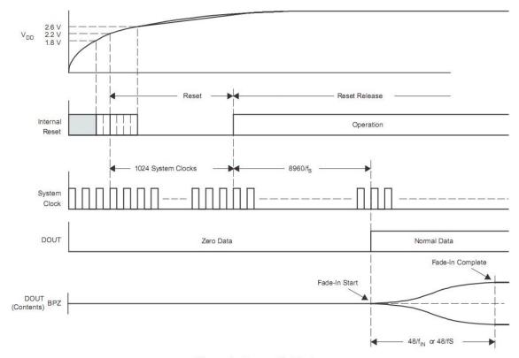
Figure 2. Power-On Timing
