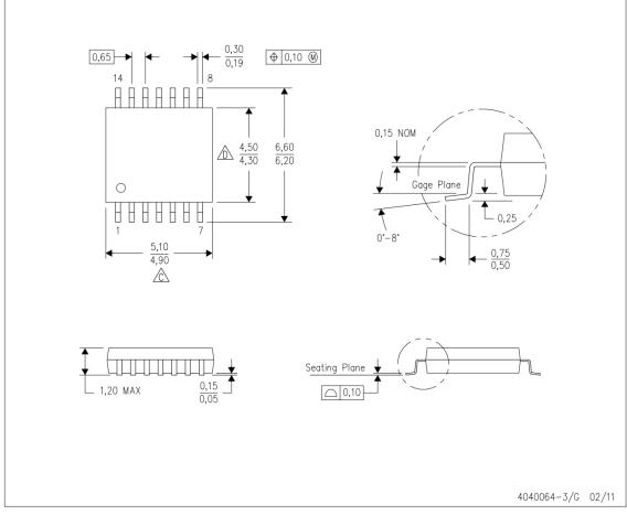
NOTES: All linear dimensions are in millimeters. Dimensioning and tolerancing per ASME Y14.5M-1994.
