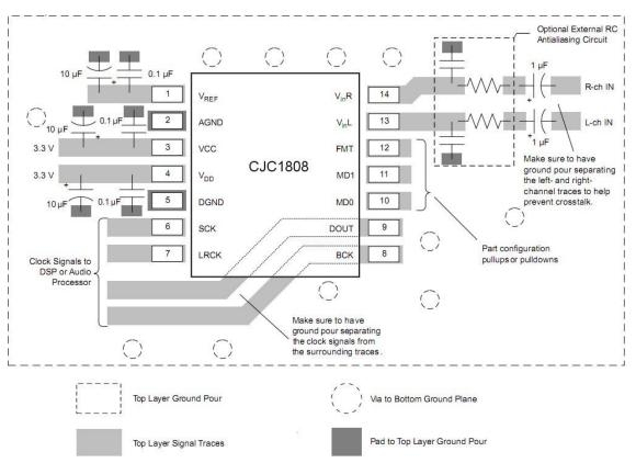
Figure 27. CJC 1808 Layout Example
