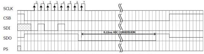
Figure 7: Conversion out sequence, Typ=d1, OSR = 4096
