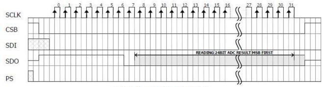
Figure 8: ADC Read sequence
