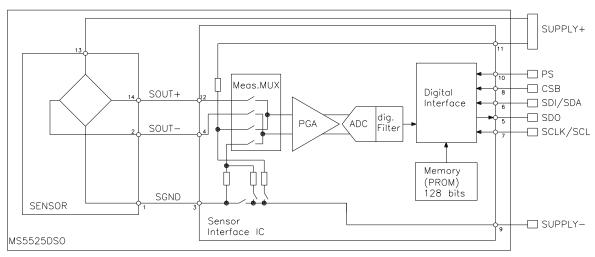
Figure 1: Block diagram of MS5525DSO
