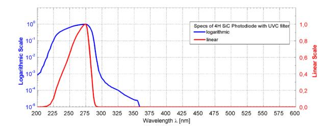
UVC-only SiC based UV photodiode A = 0,06 mm<sup>2</sup>
