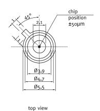
UVC-only SiC based UV photodiode A = 0,06 mm<sup>2</sup>
