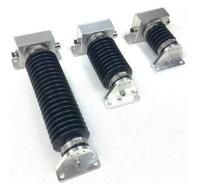
Our displacement sensor may either be used as a standalone unit or as a part of a system together with other daisy chained sensors. In standalone mode the sensor requires 24VDC supply and outputs an analogue current in the range of 4-20mA. The output signal is linearly proportional to the displacement i.e. 4mA corresponds to 0mm and 20mA represents the maximum displacement of the sensor.
