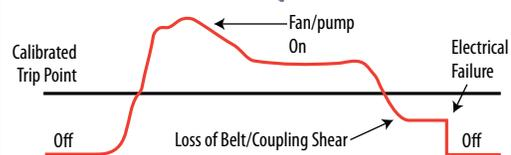
Now you can easily detect when drive belts slip, break, or pump couplings shear. In fact, a typical HVAC motor that loses its load has a reduction of current draw of up to 50%. That's why our sensors are the industry standard for status.
