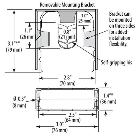
\* Terminal block may extend up to 1/8" over the height dimensions shown.
