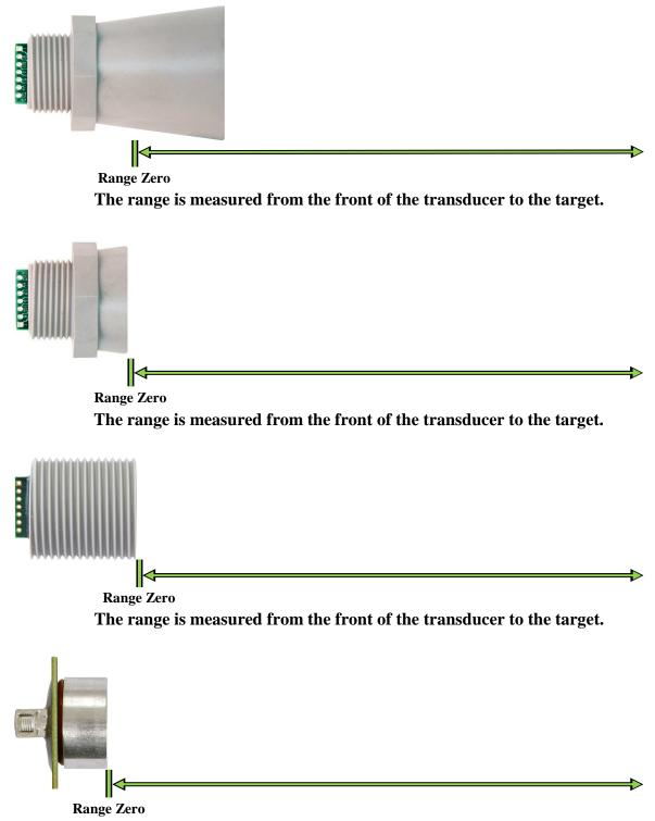
The range is measured from the front of the transducer to the target.
