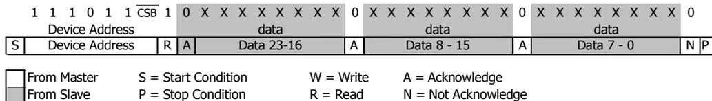
Figure 15: I<sup>2</sup>C response from MS5525DSO
