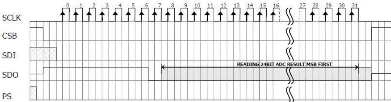
Figure 8: ADC Read sequence
