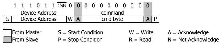
Figure 14: I<sup>2</sup>C ADC read sequence
