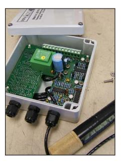
The **225-THT-1 Temperature & Humidity Sensor** is configured for measuring relative humidity and temperature in environmental control systems, where condensation or dust will commonly be encountered. A fully gasketed watertight enclosure, locking strain relief connections, and a brass sintered filter protect the electronics and sensors from environmental or mechanical damage.
